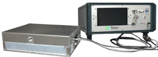
Picture of the prototype of the Mid-IR OPO compact source (on the left) and its controller (on the right)
