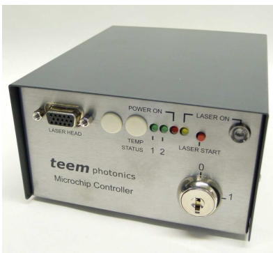
Desktop MLC-03A-DR1 for CDRH certified lasers and 100-240V AC
