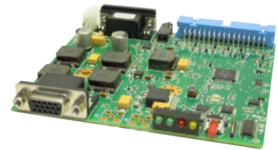
Board MLC-03A-BR1 for OEM lasers using 12V DC
