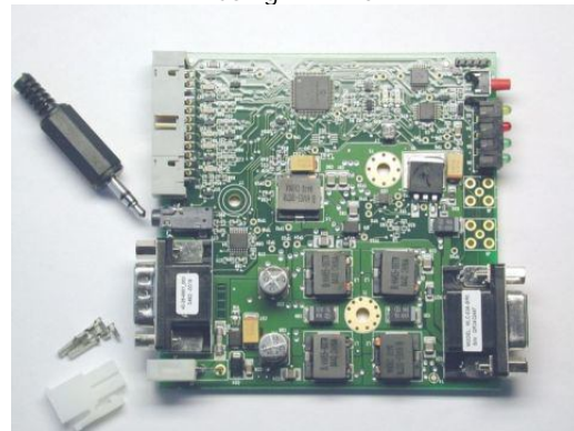
Board MLC-03A-BR0r1 for OEM lasers using 12V DC
