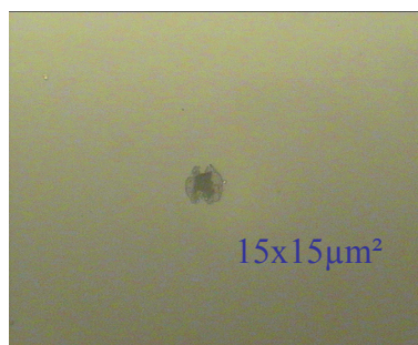
Figure 1: 266nm mark on the sample surface - x100 magnification, f=18mm
