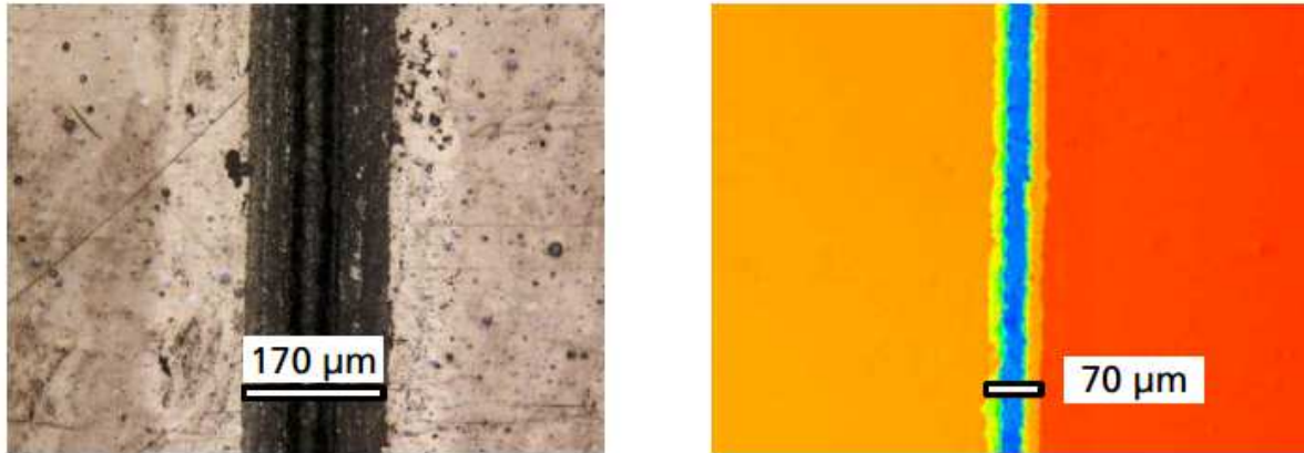
Figure 4 : backside of the sample (beam entry) : heat affected zone is only 50 \mu\text{m} on each side of the groove
